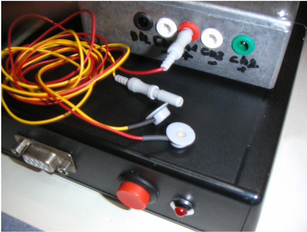
Figure 6: Electrodes connected to the ModularEEG
